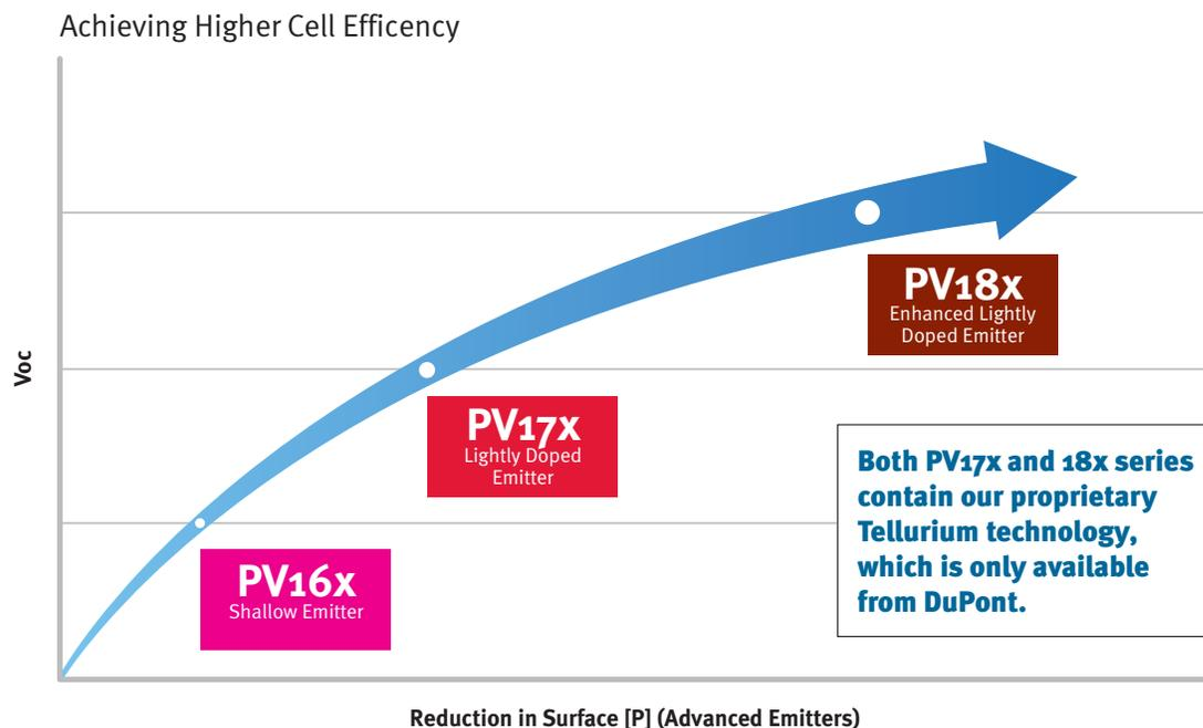
Innovative Materials Science enables contact to Enhanced LDE → Increased  $V_{oc}$  and Efficiency
